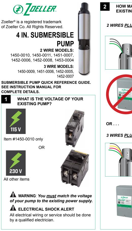
HOW MANY WIRES DOES YOUR 3 **EXISTING PUMP INCLUDE?** 2 WIRES PLUS GROUND? To Pump → WIRE + GROUND Tank No Control Box Pressure is needed Switch Wiring Diagram 3 WIRES PLUS GROUND? 3 wires plus around **3 WIRE** +GROUND То Tank Control A control box with Box the same voltage and HP as the pump is required.
