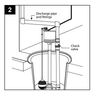
3. Make sure your hands are dry and you are not standing in water. Connect the pump to a properly-grounded, GFCI electrical outlet.
