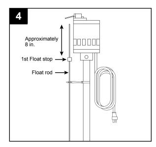
5. Slide the float rod through the hole in the pump switch.
