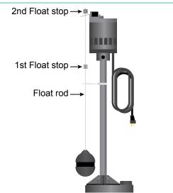
1. Assemble float rod guide and float according to included instructions.
