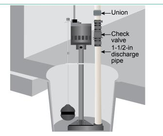
3. Install rigid 1-1/2 in. discharge pipe, union, check valve according to code.
